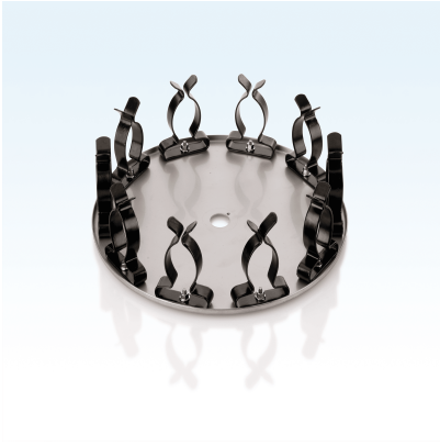
Disk with 10 clamps for tubes 28-32 mm
