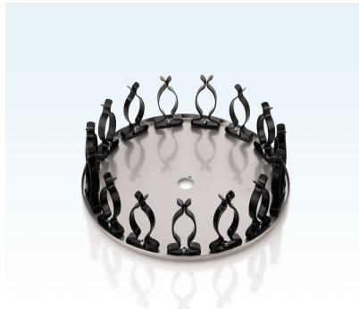
Disk with 15 clamps for tubes 22-25 mm
